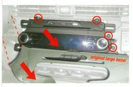
**1.** Remove the original large bezel by gently pulling away, and remove the radio with bolts as shown.
