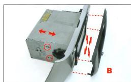
**4.** Remove the head unit and apply the self adhesive foam (A) to help support the unit, as shown.
