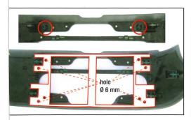
**5.** Very carefully, cut the original bezel trim using the template shown. If the original bezel cannot fit correctly due to the tabs on the rear, they can be cut off. (see figure).
