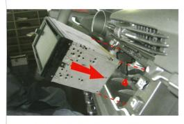
**3.** Insert the new head unit to check all interfering parts (1,2,3 above) have been correctly removed, and check alignment of unit.
